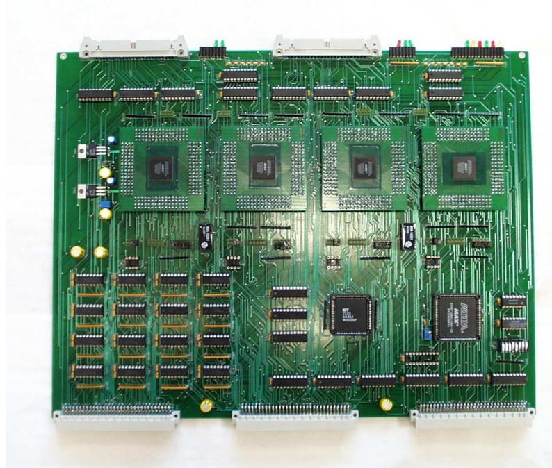
Figure 5.6: The “XYREC” trigger board
