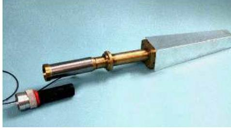
FIGURE 2.11: A fully equipped SEC module consisting of a CsI crystal, light guide and the photomultiplier tube.
