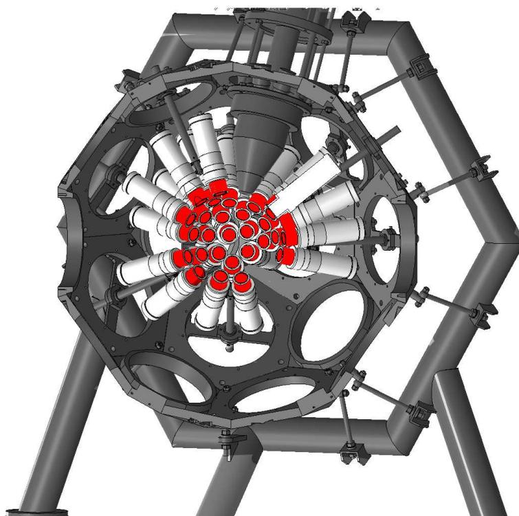
Figure 17: The EAGLE-EYE setup consists of many fast LaBr detectors that are put into the EAGLE array equipped with 16 high-efficiency HPGe anti-compton shielded spectrometers. The location of the LaBr crystals is marked in red colour. The first experiment aimed at lifetime measurement of low lying chiral band levels in  $^{128}\text{Cs}$  was performed in February 2018 with 24 LaBr detectors obtained from FATIMA and RHOSPHERE collaborations.
